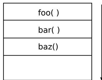
Figure 5.4: The call stack for example programs. The stack grows downward.
